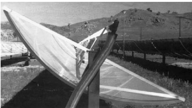
Figure 2.15 Solar thermal parabolic trough collector. (Courtesy of Caddet.)
